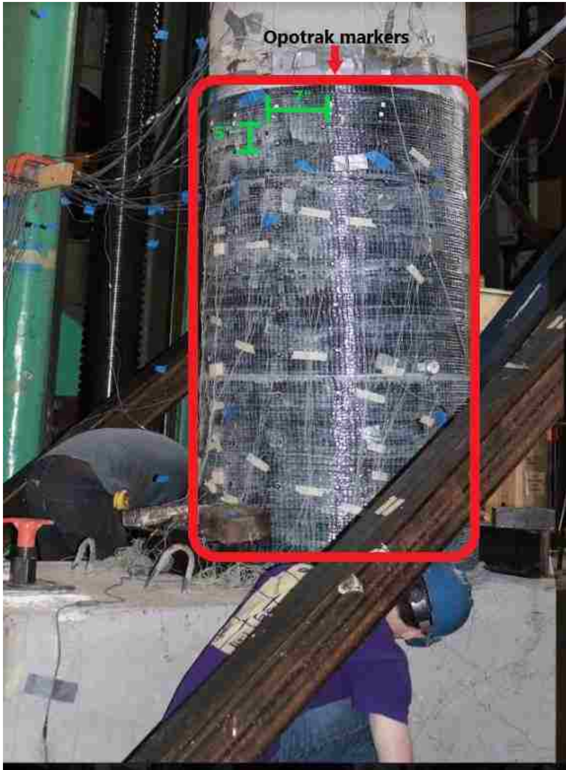
Figure 6-25. Optotrak marker grid on northwest face of specimen. Markers are all placed on CFRP within the plug region
