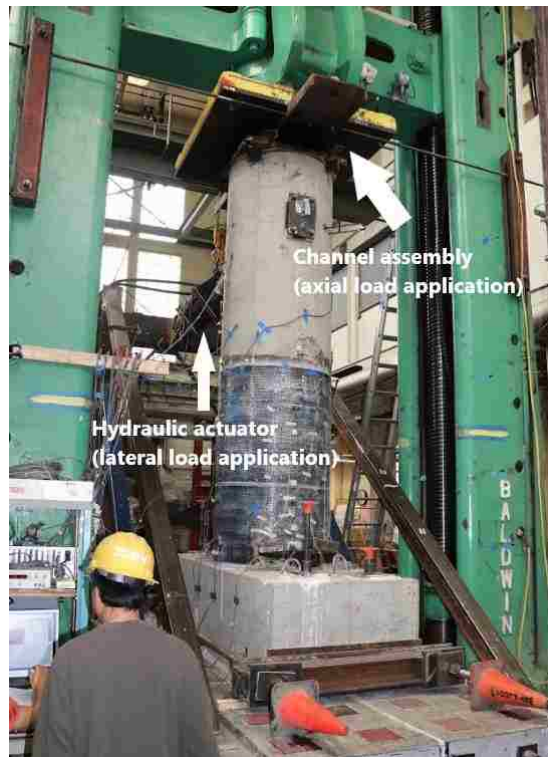
Figure 7-2. Initial position of specimen
