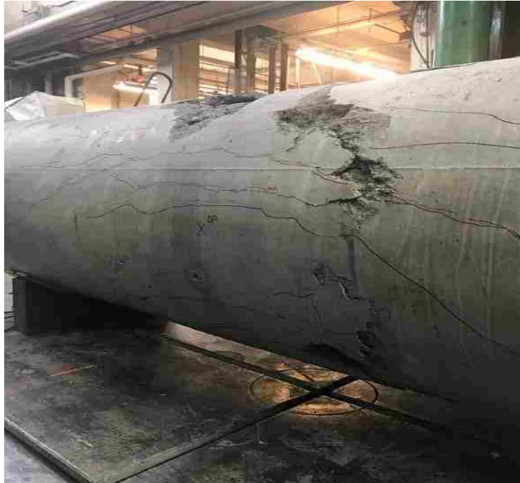
Figure 5-1. Specimen position after failure, note the angle of the cracks
