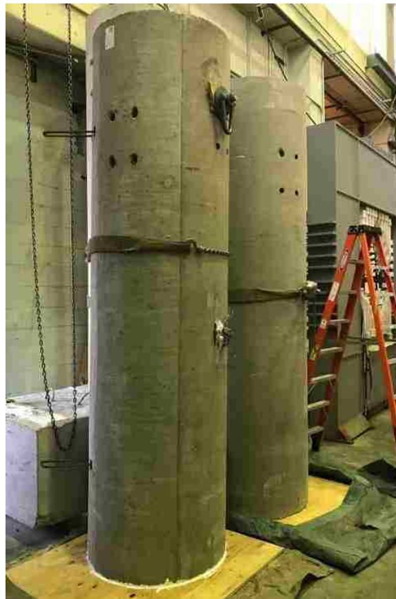
Figure 3-12. Specimen orientation prior to casting fill concrete
