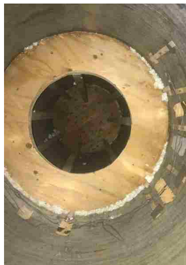
Figure 3-14. Solid disc connected to two plywood rings by 2x4 studs inside Four-point bending specimen
