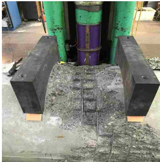
Figure 4-2. Concrete crushing and buckled strands
