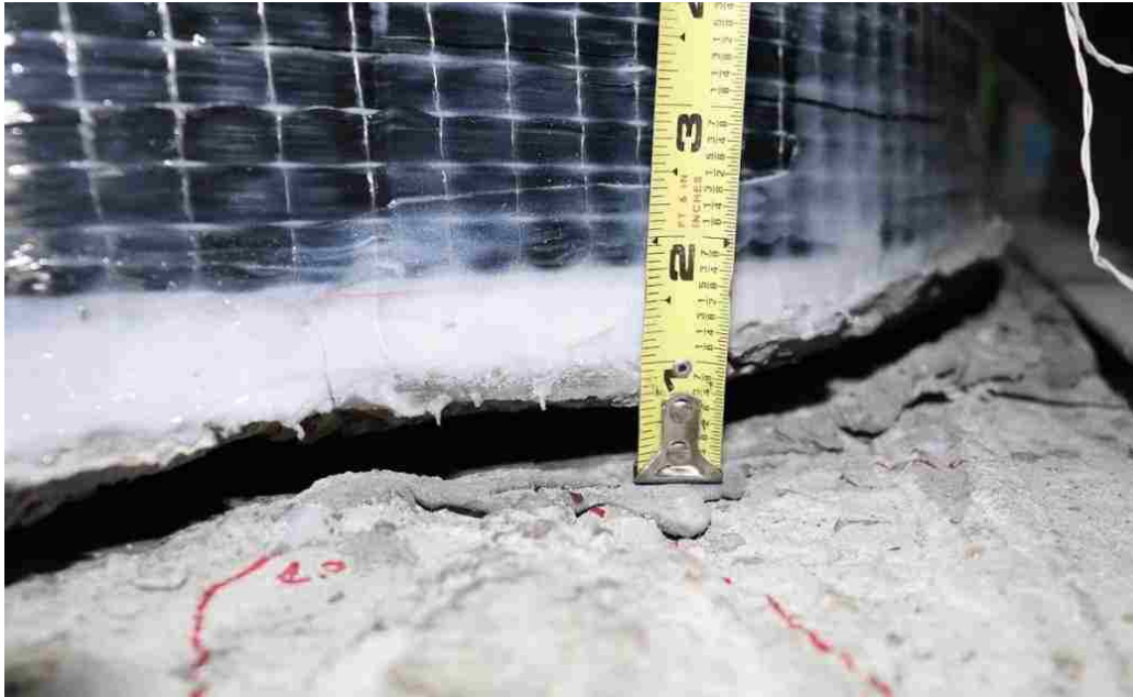
Figure 7-7. Uplift on Cycle 3 of Series 7 (+3.71%, -4.54% drift)
