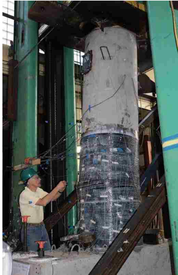
Figure 7-17. Specimen position at +8.09% drift
