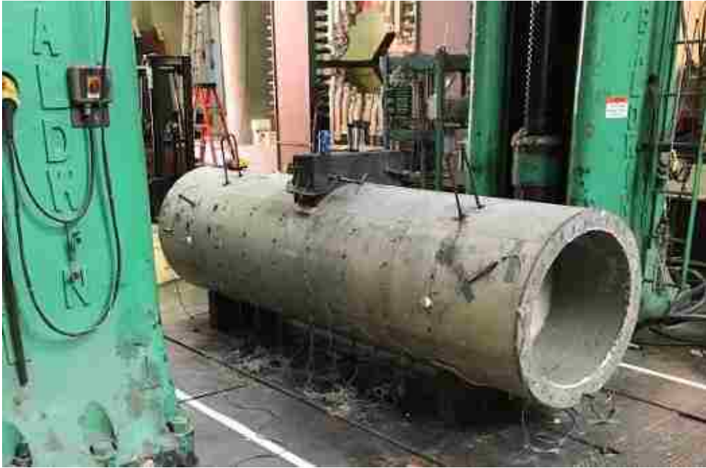
Figure 3-29. Three-point bending test optotrak and instrumentation
