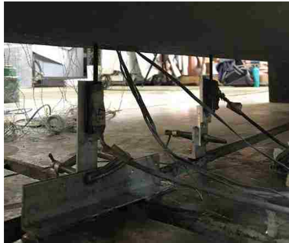
Figure 3-26. Bottom Duncan potentiometers
