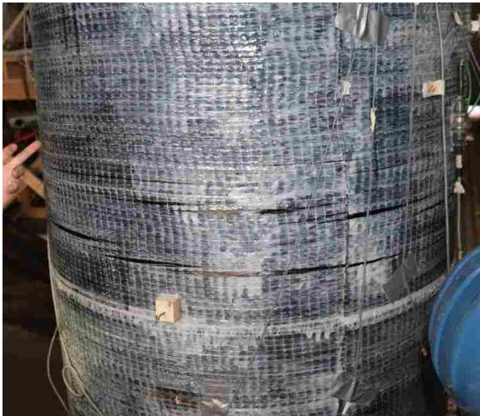
Figure 7-13. Fiber splitting on south face during Series 10
